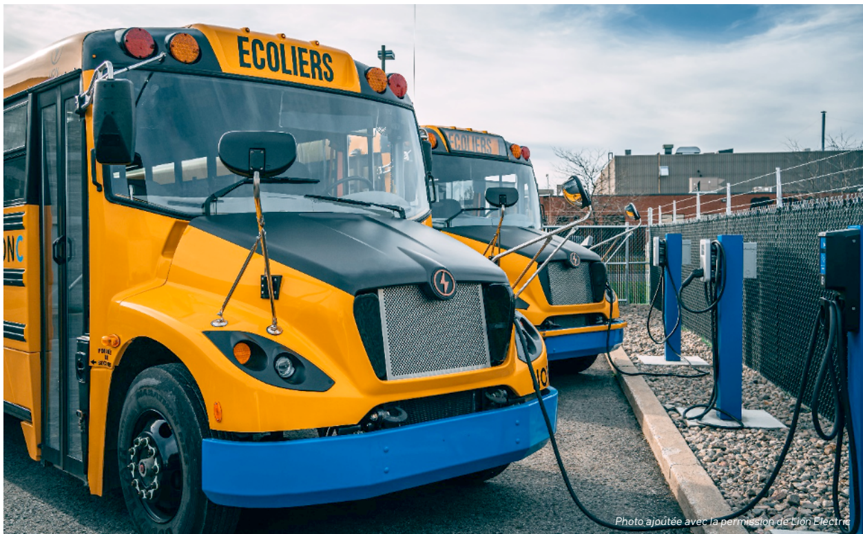
FIGURE 3 • Lion Electric buses charging at Level 2 charging stations, photo added with permission from Lion Electric
