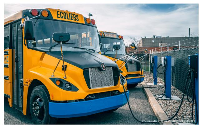
FIGURE 3 • Lion Electric buses charging at Level 2 charging stations, photo added with permission from Lion Electric
